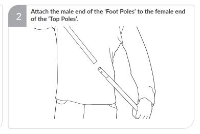
Repeat for all 3 sets of poles, ensuring all 3 connections are securely attached together.
