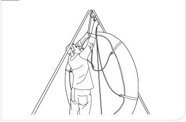
\*Warning - Never use the Hangout Pod Stand without the Strap Base Connector securely connected to all of the 3 pole legs, check before each and every use.
