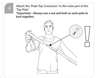
Repeat for all 3 'Top Poles' and erect upright to create a pyramid. Ensure all connections are attached and secure.
