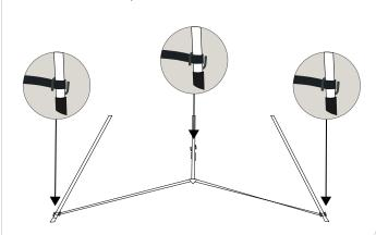
Check the Hangout Pod is hanging evenly within the center of the poles & is securely hooked onto the Stand with no twisted ropes or obstructions.
